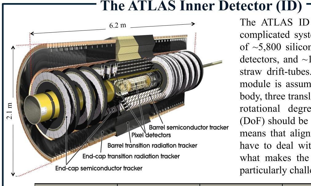
The ATLAS ID is a large and complicated system that consists of ~5,800 silicon pixel and strip detectors, and ~1000 modules of straw drift-tubes. If each silicon module is assumed to be a rigid body, three translational and three rotational degrees of freedom (DoF) should be considered. This means that alignment algorithms have to deal with ~40,000 DoF, what makes the ID alignment particularly challenging.
