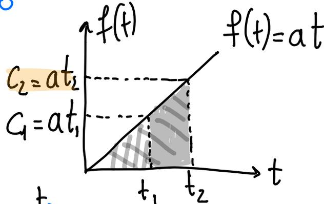
$$\begin{aligned} \int_{t_1}^{t_2} f(t) dt &= \frac{C_2 \cdot t_2}{2} - \frac{C_1 \cdot t_1}{2} = \frac{at_2 \cdot t_2}{2} - \frac{at_1 \cdot t_1}{2} = \\ &= \frac{at_2^2}{2} - \frac{at_1^2}{2} = \frac{1}{2} at_2^2 - \frac{1}{2} at_1^2 \end{aligned}$$
