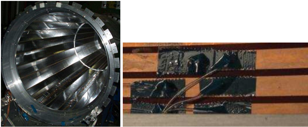
Figure 5.8: The set of mylar strips (Left), high voltage connections of the first three inner copper strips (Right).
