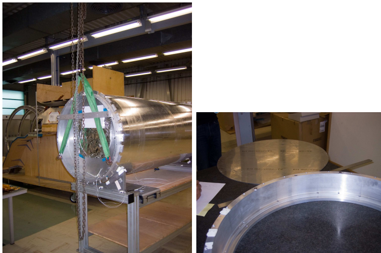
Figure 5.14: Dismantling the HARP flange (Left), fixing the adaptative ring (Right).
