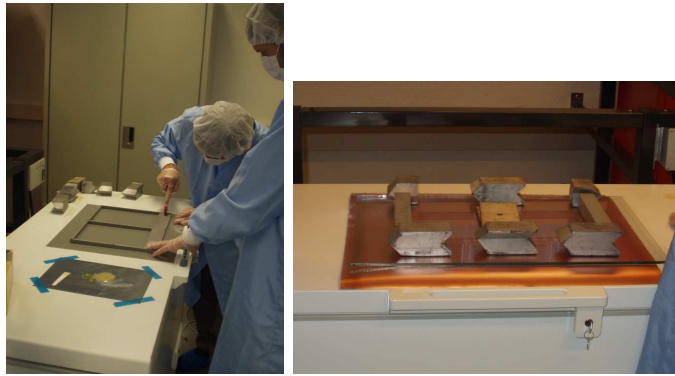
Figure 7.10: Spreading glue on the guard ring (Left), drying with weights (Right).
