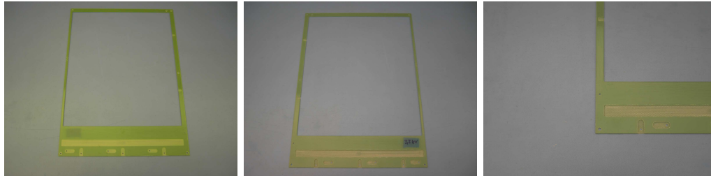
Figure 6.15: Cathode face of a frame (Left), anode face of a frame (Middle), detail of the service area of the anode face (Right).
