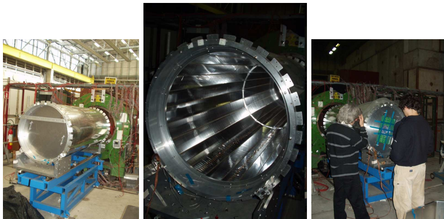
Figure 7.22: HARP chamber with the endcap (Left), the field cage (Middle), fixation of the detector flange (Right).
