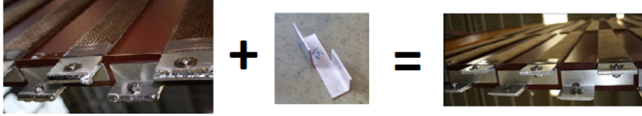
Figure 30: First prototype of the BabyMIND magnet.
