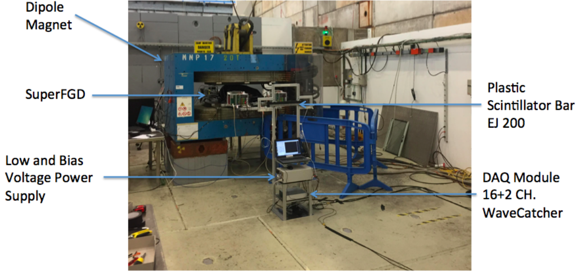
Figure 12: Photo of S_3 counter in front of SuperFGD in the testbeam area of the CERN PS.
