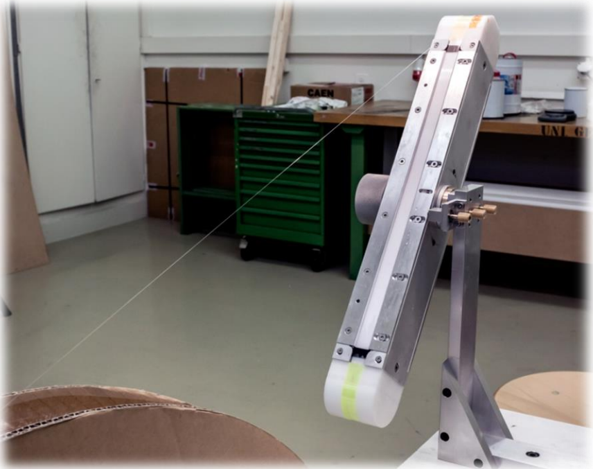
3 to 5 layers of 0.25mm scintillating fibers
