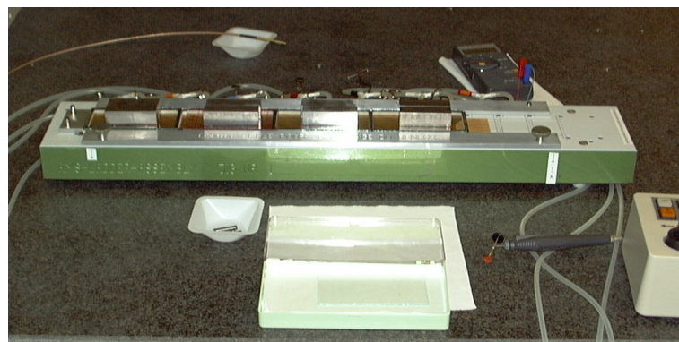
Figure 5.13: Lead blocks on glass plates are placed on the reinforcement.
