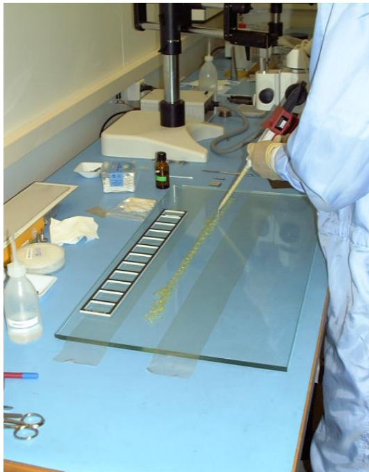
Figure 5.8: Reinforcement gluing: Araldit 2011 is dispensed on a large glass plate.
