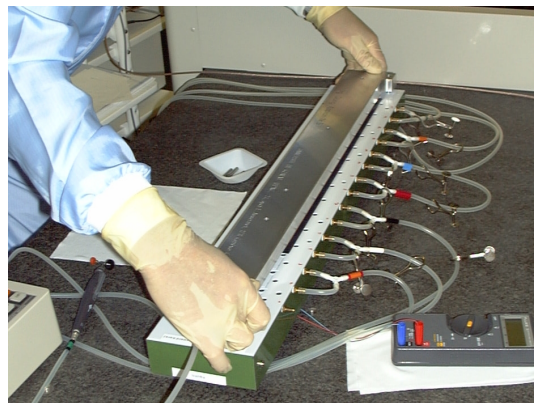
Figure 5.7: After glue deposition, the transfer jig is placed on the silicon jig.
