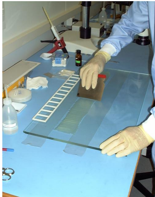
Figure 5.9: The glue is spread with a spatula, the glue thickness will be close to 80\ \mu\text{m} .
