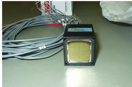
Figure 3.6: One of the photomultipliers adopted for FAST. The photocathode, with its 16 pixels ( $4 \times 4$ ), is visible in the front.
