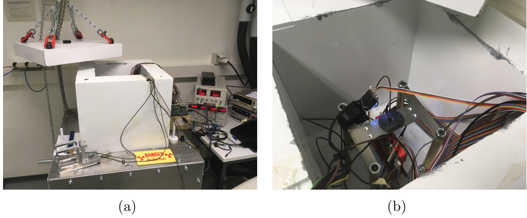
Figure 8.4: Experimental setup of the annihilation photon detection. A lead box for radiation protection (a) and the inside of the box (b). The two boards with the metal support structure were fixed and monitored by USB cameras after closing the cover of the box.
