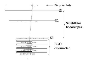
**Fig. 1.** ATIC detector response to a high energy event (~ 5 TeV incident energy) and the reconstructed incident particle trajectory (nearly vertical line) in the ATIC detector system.
