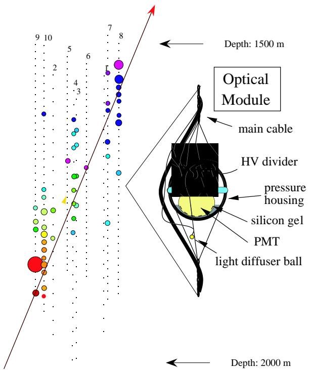
**Fig. 1.** The AMANDA-B10 detector as of 1997. Each dot represents an optical module. The modules are separated by 20m on the inner strings (1-4), and by 10m on the outer strings (5-10). Shown is an experimental neutrino event. The size of the circles indicates the amplitude of each detected signal the color indicates the time of the photon's arrival. Earlier times are in red, later in blue. The arrow indicates the reconstructed track of the up-going muon.
