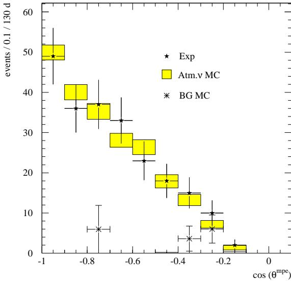
**Fig. 3.** Distribution of the cosine of the reconstructed zenith angle for analysis-B. Shown are the experimental data points with the MC expectations for the atm. $\mu$ -background and the atm. neutrino simulation. The MC includes effects from neutrino oscillations and local hole ice defects. Note that the BG simulation is limited by statistics.
