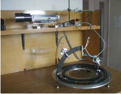
Figure 1. Picture of the spectro-gonio-reflectometer out of its dark vessel. From the top left one see the D2 Lamp (black), the spectrometer (grey) out of which the grey fiber cable is driven and fixed on one arm of the goniometer; on the other arm on the left the PMT is fixed. On the right is shown a schematic drawing of the measurement principle with notations.
