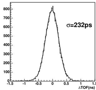
Figure 3. Overall resolution of TOF
