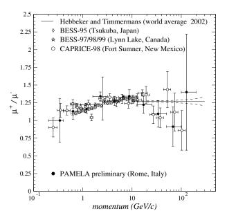
**Figure 2.** Preliminary result on the all-particle charge ratio measured by PAMELA during the ground test.
