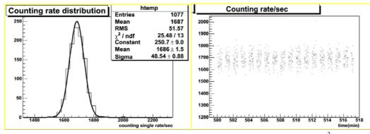
**Figure 3.** Rate distribution observed in Sierra la Negra with a mean value of 1686 part/ s/  $m^2$ . The typical dispersion rms/mean was lower than 3%. Small variations in the counting rate can be observed (right).
