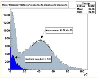
**Figure 1.** Water Cerenkov detector response to muons and electrons. The deposited charge ratio from muons and electrons is 41.7/3.5 = 12, which is consistent with muon energies around 1 Gev crossing 70 cm of water and electons with energies around 10 Mev.
