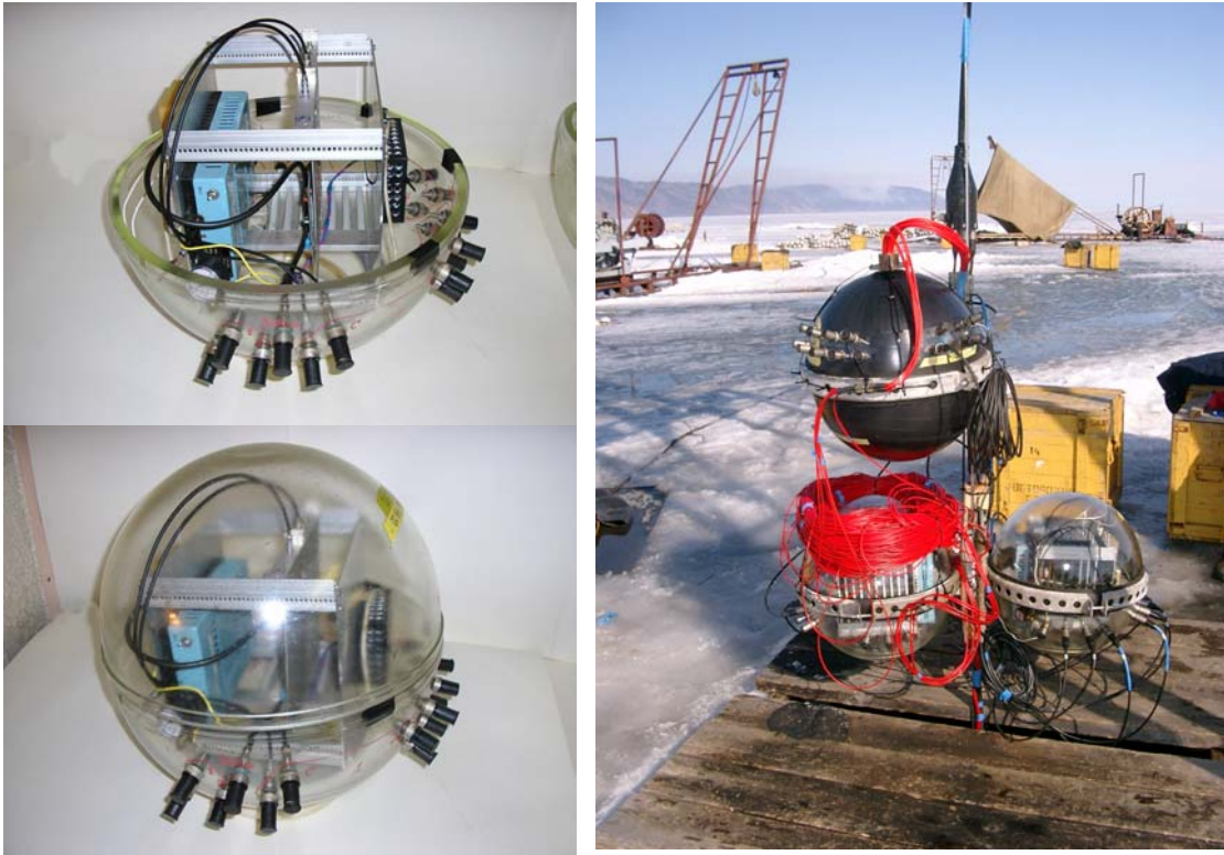
Figure 3. Left: Light source, electronics and pressure housing. Right: Light source module fixed at underwater cable ready for deployment. One can see optical fibers attached to the light source module. To avoid stray light the module is blackened.
