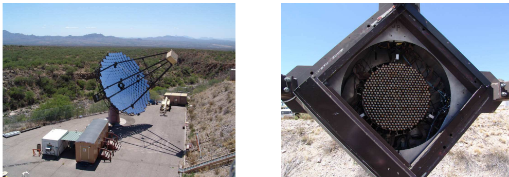
Figure 1. Left: VERITAS Telescope 1. Right: The 499 pixel PMT camera.
