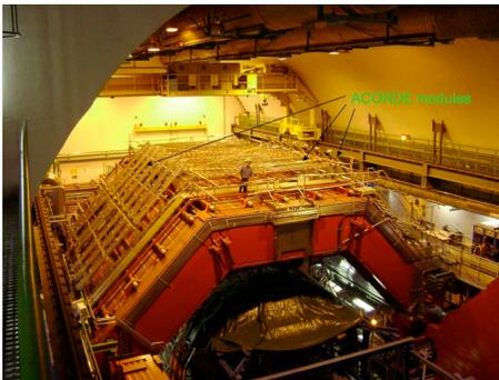
Figure 2: Photo of the ACORDE scintillator module array on the upper faces of the magnet yoke, in the ALICE pit, located in the P2 site, of the LHC ring, 60m underground. There are twenty modules on each one of the three upper phases.
