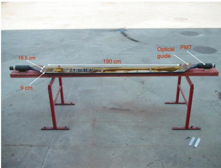
Figure 1: ACORDE module unit. This device includes two scintillator counters overlapped, each with  $190 \times 20 \text{ cm}^2$  effective area, and 10mm thickness, plus two PMTs placed on the ending side of each scintillator, with optic guide and iron magnetic shielding. All components are attached to an aluminum structure, assembling a 40kg robust box.
