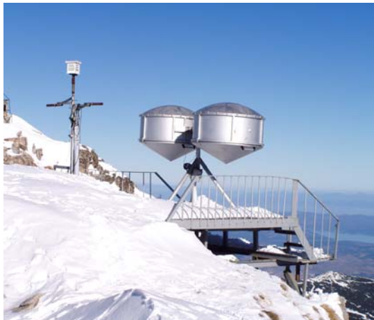
Figure 2: Ice Lake experiment mirrors - prototype for Kartalska filed gamma telescope
