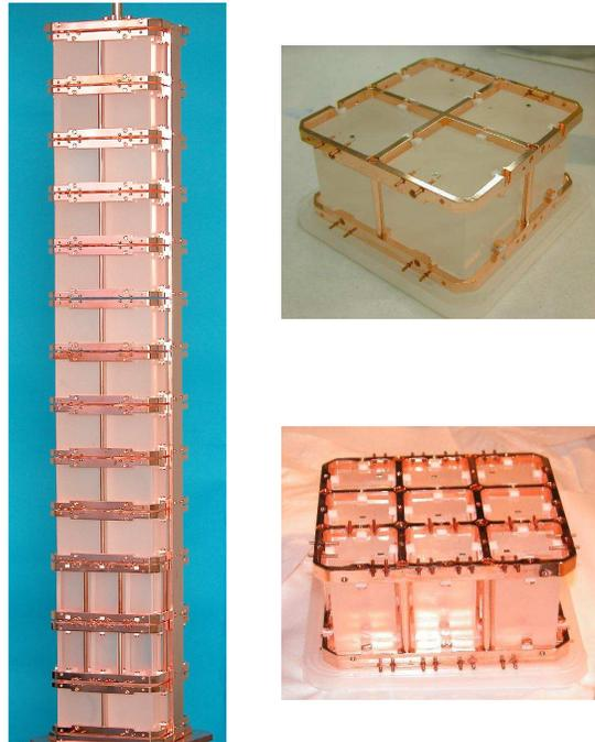
Figure 1: CUORICINO array (left) and details of the planes hosting the  $5 \times 5 \times 5$  cm<sup>3</sup> crystals (top right) and  $3 \times 3 \times 6$  cm<sup>3</sup> crystals (bottom right)
