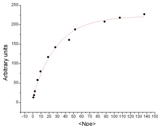
Figure 4: SiPM response plotted versus the PMT response when the fibers were excited with UV-LED light. The saturation of the SiPM follows the predicted behaviour (solid line).
