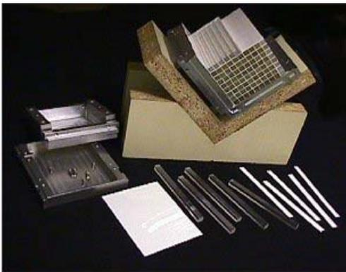
Fig. 2: MEGA Calorimeter module. [6]
