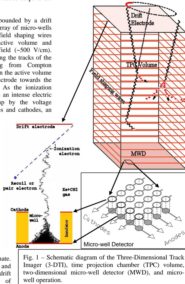
Fig. 1 – Schematic diagram of the Three-Dimensional Track Imager (3-DTI), time projection chamber (TPC) volume, two-dimensional micro-well detector (MWD), and micro-well operation.
