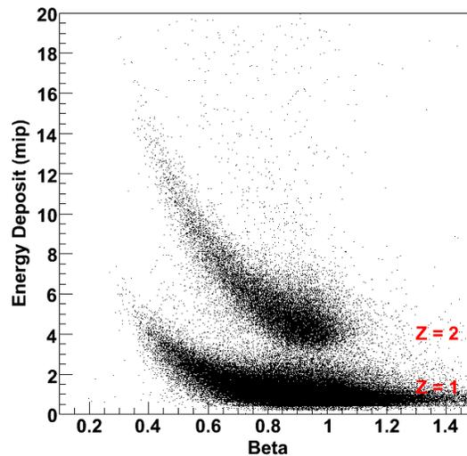
Figure 7: Charge bands for flight data measured by one photomultiplier in a S2 scintillator
