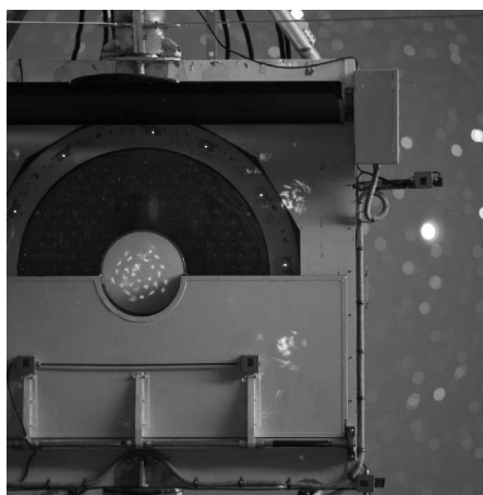
Figure 3: Light-spots of 30 mirror tiles defocused to a pre-calculated pattern on a reflector at the center of the PMT camera.
