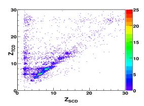
Figure 1: SCD versus TCD charge for events passing through the full TCD-TRD-SCD stack. Identically identified charges lie along the diagonal, with B, C, N, and O most prominent. All remaining events lie in the reasonable region of lower SCD than TCD charge. Events along the TCD-identified C and O lines correspond to charge-changing interactions within the instrument.
