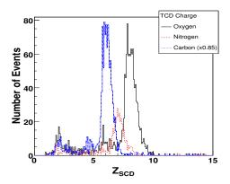
Figure 3: TCD-identified O, N, and C with good tracks in the TCD and SCD active areas correspond to their SCD-determined charge. TCD O fragmenting to N and C events are also visible. The latter are more prevalent due to resonance at alpha emission.
