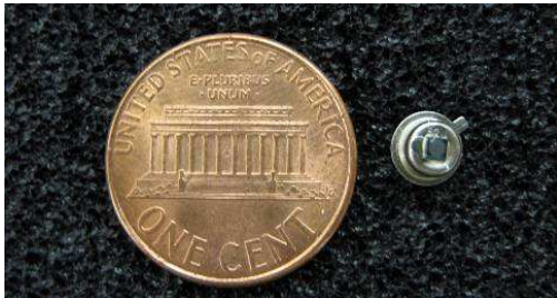
Figure 1. A 1 \times 1 \text{ mm}^2 active area Si-PM (a US one cent coin is shown for scale).
