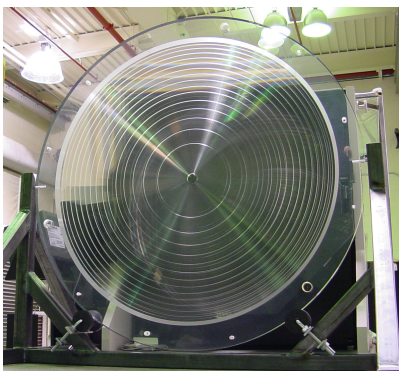
Fig. 2 A prototype model of the Fresnel lens of the JEM-EUSO telescope with a diameter of 1m.
