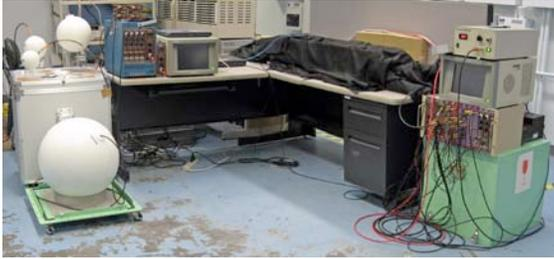
Figure 1: Experimental apparatus for measurement of cosmic ray neutron spectra. (Left) Bonner multi-sphere spectrometer (right) scintillation counter.
