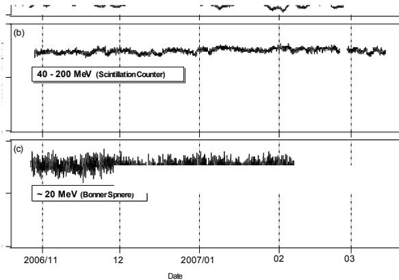
Figure 4: Time dependence of neutron flux measured at Mauna Kea Summit. (a) atmospheric pressure measured at Subaru Telescope building (b) neutron flux in 40 – 200 MeV range measured by scintillation counter (c) neutron flux at around 20 MeV measured by Bonner sphere detector.
