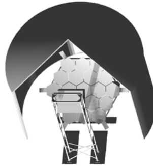
Figure 3: A drawing of the prototype Tower Detector mirror on its stand in the building where it has been deployed. The cluster box is also shown. The mirror stand is designed to also hold the full size mirrors.
