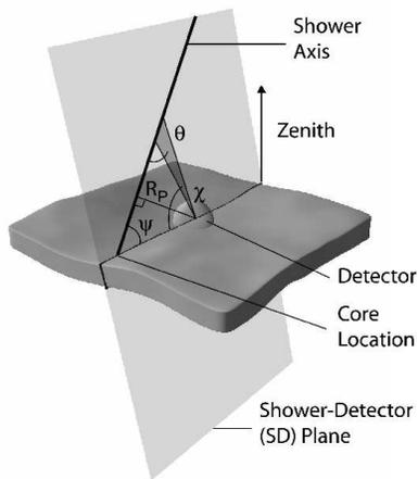
Figure 1: The geometry of reconstruction for a monocular air fluorescence detector
