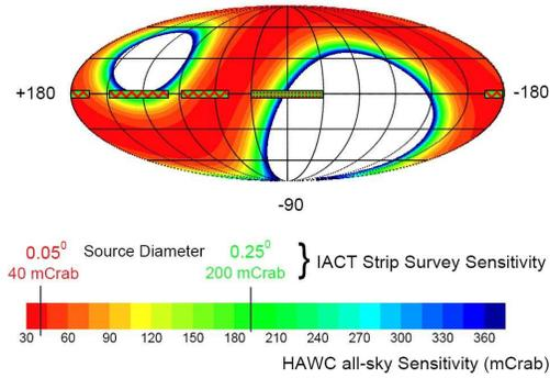
Figure 3: Flux limits for HAWC versus the HESS sky survey and the proposed VERITAS sky survey over the next two years. HAWC is assumed to be located in Mexico ( $19^\circ$ N). IACT sensitivity is shown for point (red) sources and for sources extended by  $0.25^\circ$  (green). A crab-like spectrum is assumed. The HAWC limits will be lower for harder sources.
