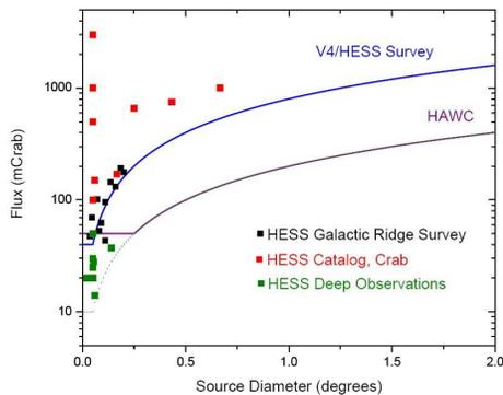
Figure 5: Comparison of  $\gamma$ -ray sensitivity between the IACT and HAWC 2 year sky surveys as a function of the source angular diameter. The HESS detected Galactic sources are shown as well as the Milagro source in the Cygnus region.
