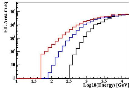
Figure 1: HAWC effective area versus gamma-ray energy for three different levels of trigger multiplicity (20(upper red line), 80(blue line) and 200(lower black line) PMT trigger) for a zenith angle  $< 30^\circ$  after applying the cosmic ray background rejection cut and requiring a reconstructed direction within  $1^\circ$
