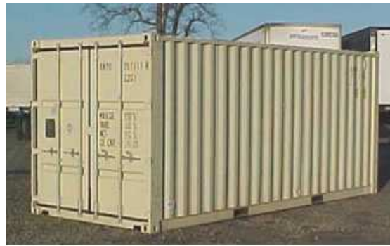
Figure 3: 20 \times 8 \times 8 \text{ ft}^3 “Connex box” (shipping container).
