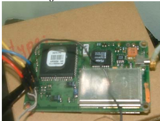
Figure 7: Embedded GPS receiver used to attach a precise time tag to each event that passes the L2 trigger at the EAS-UAP array.
