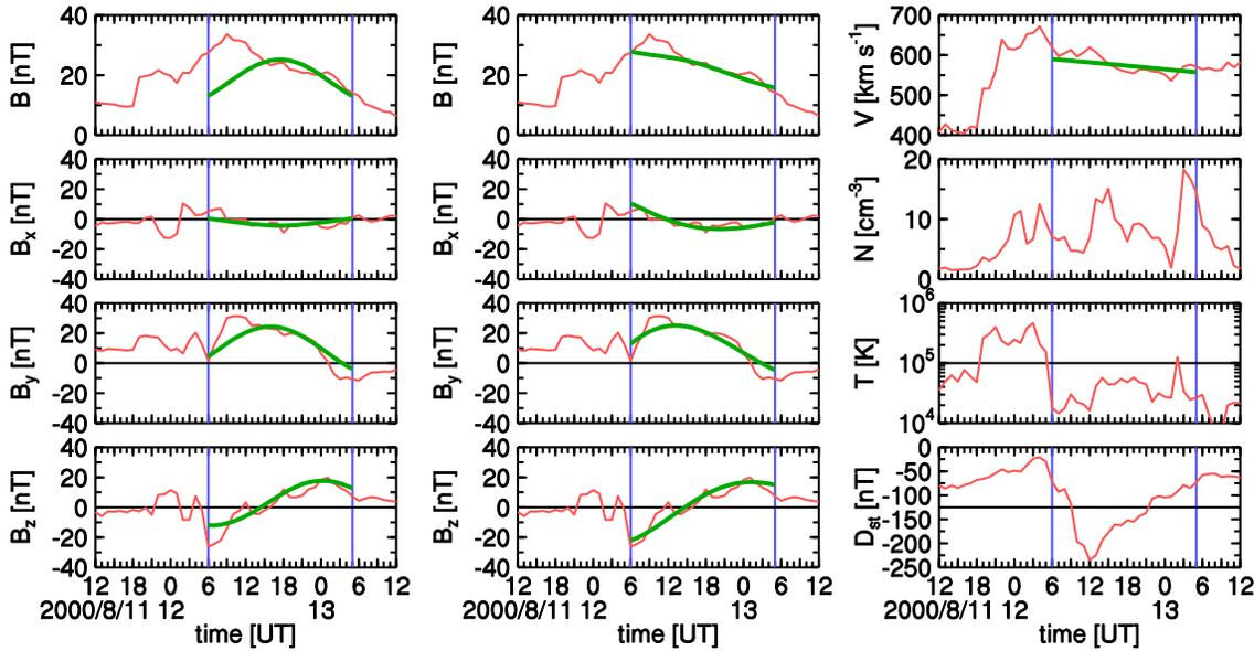
Figure 3: Magnetic field magnitude  $B$ , and components  $B_x$ ,  $B_y$ ,  $B_z$ , for circular (left column) and elliptic (central column) cylindrical clouds. Speed  $V$ , density  $N$ , proton temperature  $T$  of plasma inside the cloud and  $D_{st}$  index (right column). Thin line (red) is the experimental data, bold line (green) the simulated data. Vertical thin lines (blue) are the cloud's boundaries.
