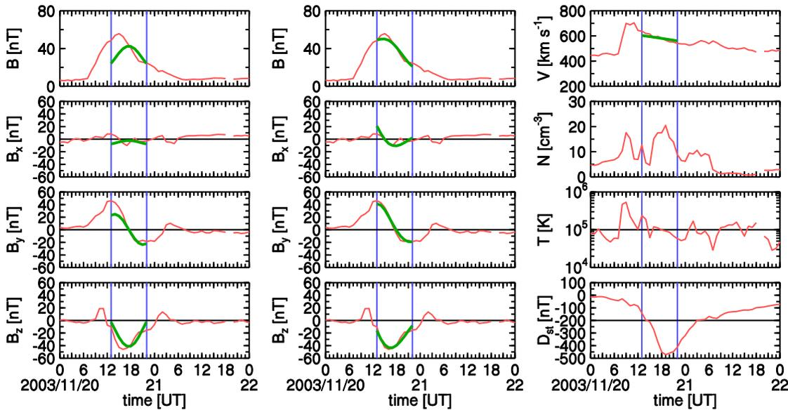
Figure 5: Magnetic field magnitude  $B$ , and components  $B_x$ ,  $B_y$ ,  $B_z$  for circular (left column) and elliptical (central column) cylindrical clouds. Speed  $V$ , density  $N$ , proton temperature  $T$  of plasma inside the cloud and  $D_{st}$  index (right column). Thin line (red) is the experimental data, bold line (green) the simulated data. Vertical thin lines (blue) are the cloud's boundaries.
