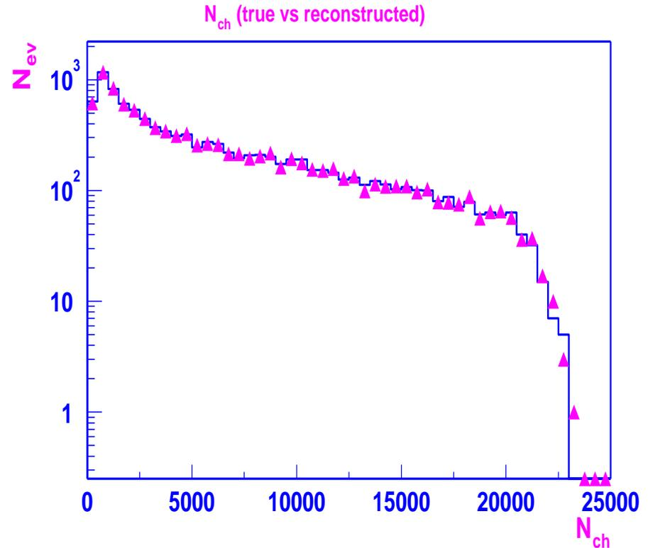
generated vs estimation from pixel counting, **no track reconstruction!**
