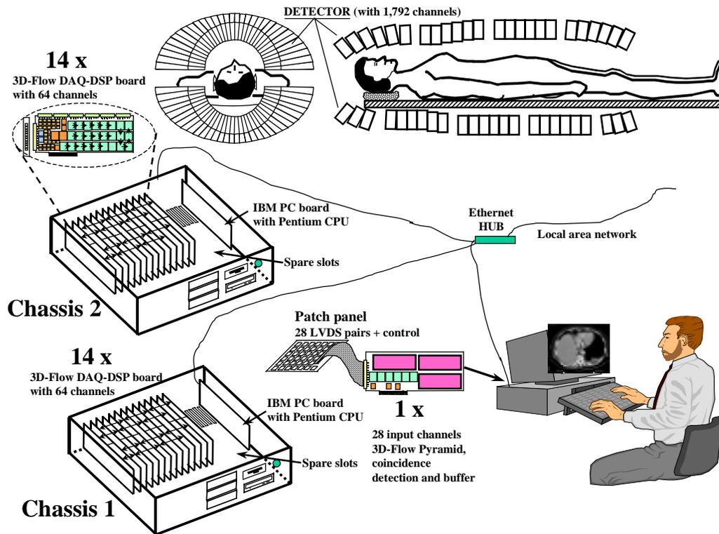
Figure 10. Layout for the hardware assembly of the 3D-CBS.
