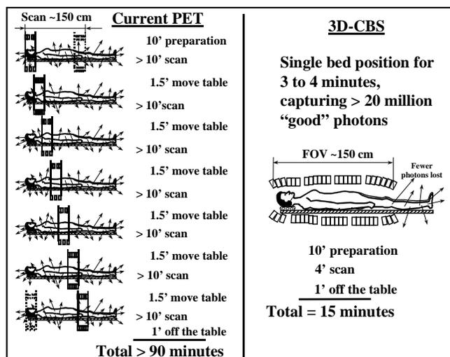
Figure 2. The current PET (figure at left) with short (< 25 cm) axial FOV (the length of the detector) requires  $\geq 7$  scanning table positions,<sup>2</sup> each longer than 10 minutes, to cover about 150 cm of the body and record more than 20 million data of photons in time coincidence. The 3D-CBS (figure at right) with a longer axial FOV (~150 cm) and with more efficient electronics, can capture > 20 million data from photons in time coincidence in < 4 minutes.
