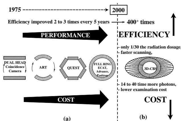
Figure 16. The evolution of positron imaging systems (original source of the figure [20], on the left). Section (a) shows the evolution of the PET using the past and current approach, while Section (b) shows the improvements achievable with the new 3D-CBS described in this document.
