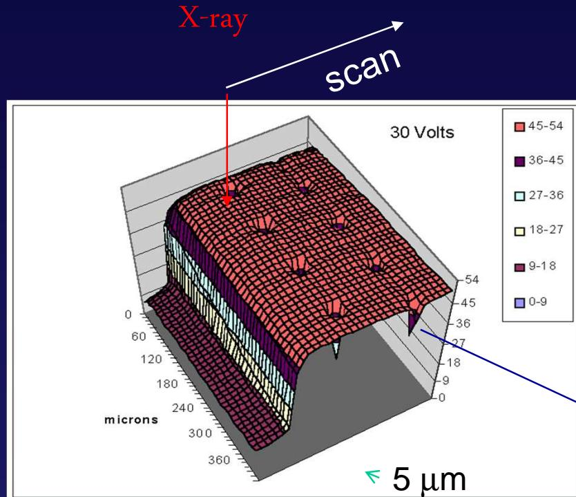
12 KeV X-ray scan at ALS, Berkeley, in 2  $\mu\text{m}$  steps, of a 3D, n bulk and edges, 181  $\mu\text{m}$  thick sensor.
