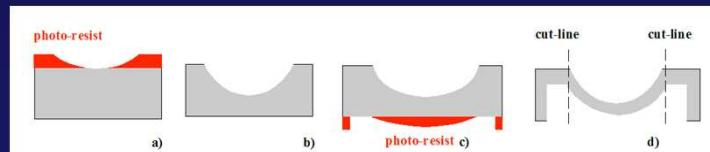
Principle of gray-tone technology: The 3-D resist profile, a) and c), is directly transferred into silicon topography, b) and d).
