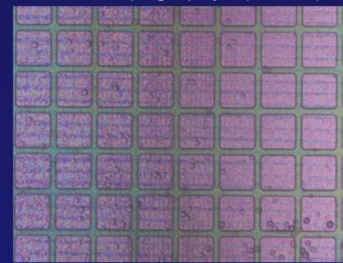
Top-view optical micrograph of a pixel array on a curved detector(pixel dimensions 150 x 150  $\mu\text{m}$ ).
