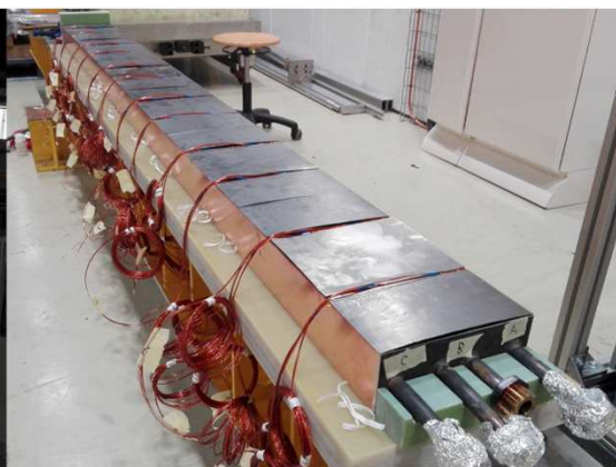
HIPed CuCr1Zr cooling plate test bench
