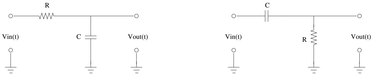
Figure 11: Low-Pass or integration circuit on the left and High-Pass or differentiation circuit on the right.
