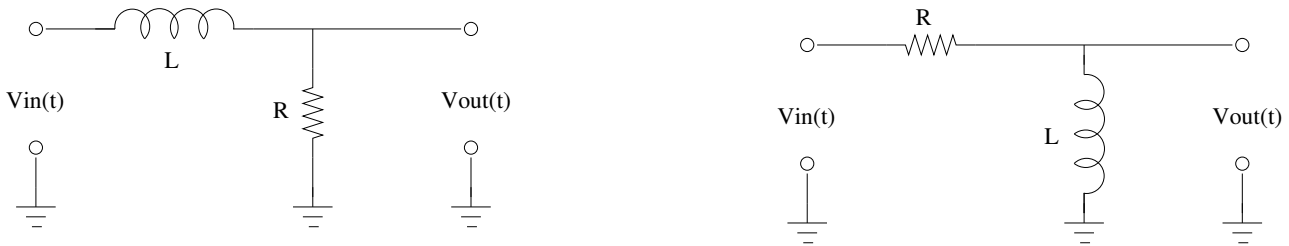
Figure 12: Low-Pass RL circuit on the left and High-Pass RL circuit on the right.
