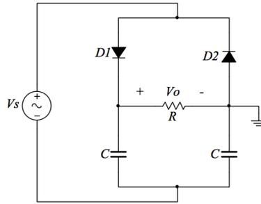
Figure 7: Pompe de charge ("voltage doubler circuit").
