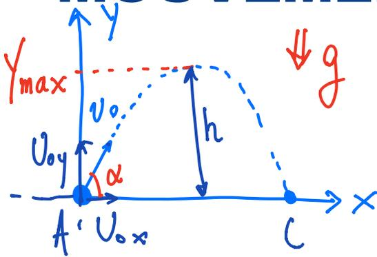
$$h = Y_{\max} = \frac{v_{0y}^2}{2g} = \frac{v_0^2 \sin^2 \alpha}{2g}$$
