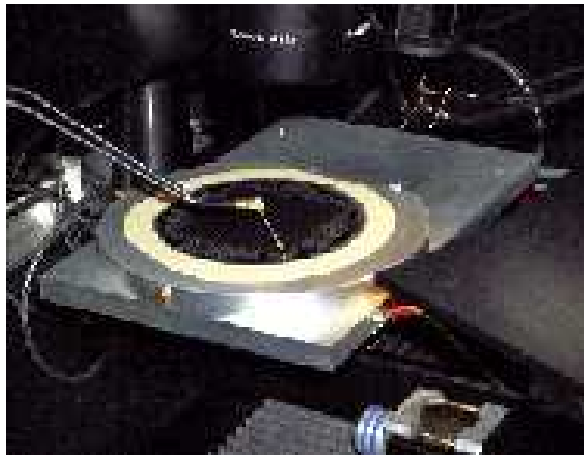
Figure 4.1: A detector on the probe-station chuck.
