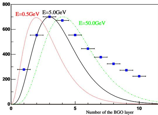
**Figure 3:** The typical shape of the deposited energy in the BGO calorimeter when  $200A \cdot GeV/c$  Fe ions made a normal incidence on the ATIC at the center.
