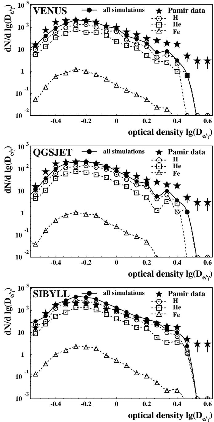
Figure 3: Measured optical density spectrum ( $ST = 11.5 \text{ m}^2 \text{ yr}$ ) of single particles in the working layer (12 c.u.) of the Pamir experiment ( $N_{e,\gamma} = 1469$ ) compared with the simulated spectra of different primaries normalized to the measured exposure time for three different interaction models.
