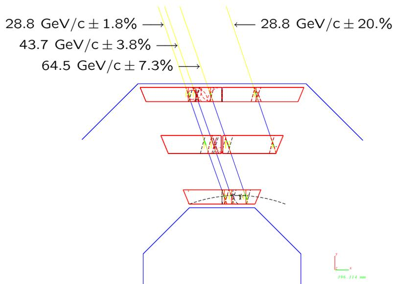
Figure 2: A four muon event.- In the three chamber layers, track segments reconstructed for all ambiguities are shown. Fully reconstructed tracks are drawn for the surviving ones only.
