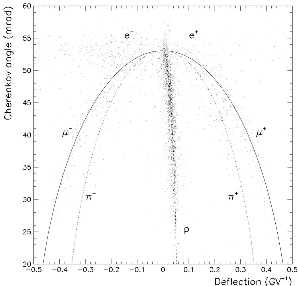
Figure 1: Cherenkov angle as function of deflection in the spectrometer for the data observed in this experiment. The rigidity is  $1/\text{deflection}$ . The total number of events included in the plot is 8147.
