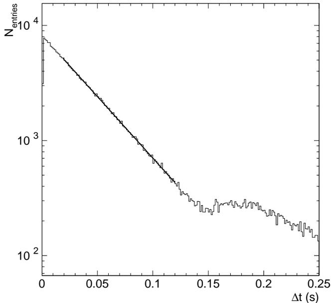
Figure 1: Distribution of the time between triggered events  $\Delta t$ . This figure shows the fit for data taken during day 120.
