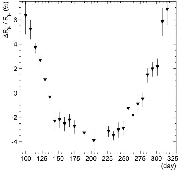
Figure 2: The measured relative variation of the trigger rate around its mean  $\Delta R_\mu / \langle R_\mu \rangle$  as a function of day number, for the 225 days used. The data is sorted in bins of 7.5 days.
