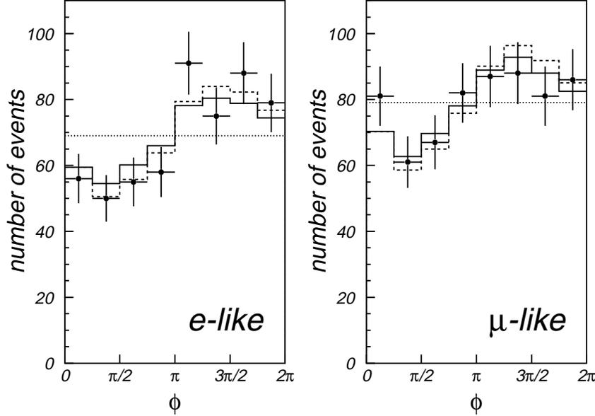
Figure 2: Azimuthal distribution of e-like and  $\mu$ -like events. Closed circles show the data, solid histograms show the expectation based on (Honda et al. 1995) and dashed histograms show the expectation based on (Lipari et al. 1998).  $\phi=0, \pi/2, \pi$  and  $3\pi/2$  are corresponding to the events going to north, west, south and east.
