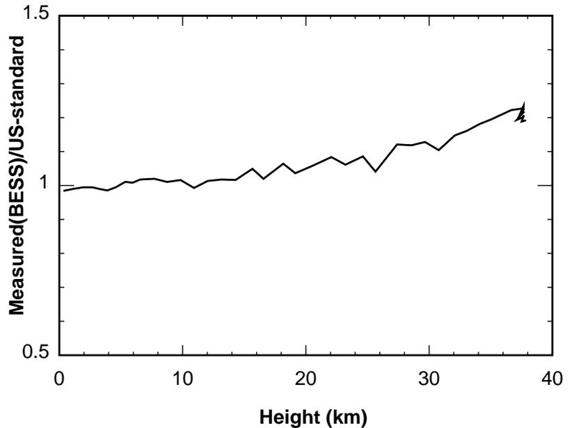
Figure 3: The atmosphere pressure ratio: measured and US-standard at high altitude. The measurements were made by on board pressure gauge and GPS position sensor in 1997 BESS flight at Lynn Lake (Orito, S. 1998)
