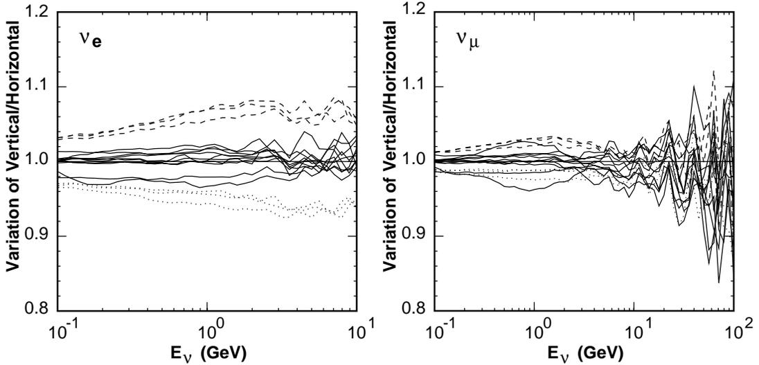
Figure 4: The variation of (vertical flux)/(horizontal flux) for  $\nu_e$ . Dashed lines are for the atmospheric model with 10 % larger scale height and dots for 10 % smaller scale height. Each 3 line stands for high, mid, and low primary flux model. Other lines near (vertical flux)/(horizontal flux)  $\sim 1$  are variation for the interaction model variation.
