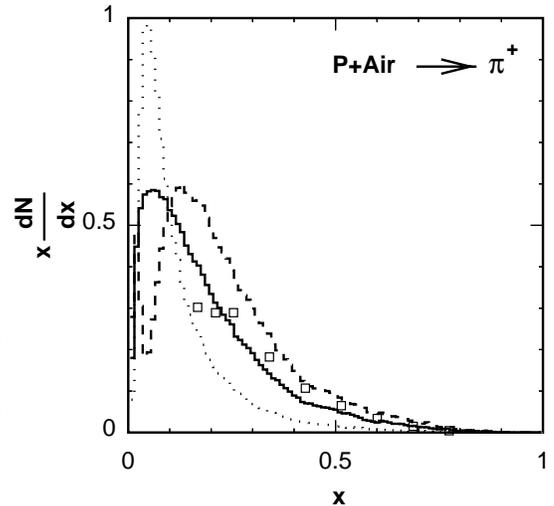
Figure 2: Example of modification of interaction model for secondary particle energy spectrum with experimental data from Eichten, T., et al., 1972.
