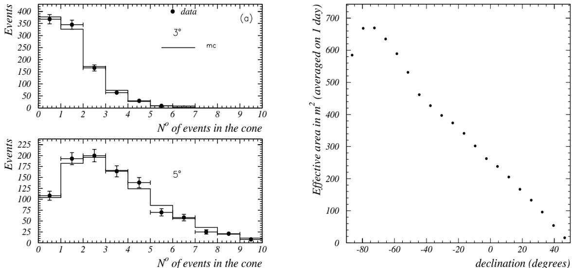
**Figure 1:** (a) Distribution of the number of events inside cones of  $3^\circ$  and  $5^\circ$ . (b) MACRO effective area as a function of declination averaged on 1 day for high energy events ( $E_\mu \geq 10$  GeV).
